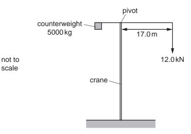
The counterweight has a mass of 5000 kg. The crane is required to lift a load of 12.0 kN and the horizontal distance from the pivot to the load is 17.0 m.
